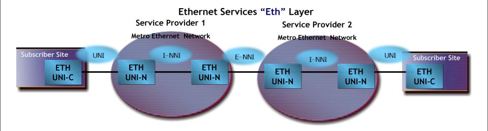
UNI: User Network Interface, UNI-C: UNI-customer side, UNI-N network side NNI: Network to Network Interface, E-NNI: External NNI; I-NNI Internal NNI
